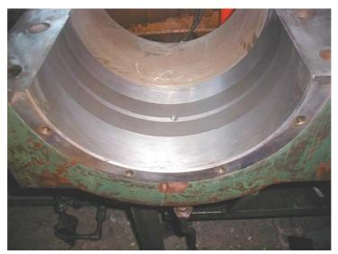
In a steel plant the repair of a broken spool reductor with a weight of 40 t would have taken up 10 days by using the conventional way of welding. By using the repair technology of MultiMetall combined with the PolymerMetal MM-metal SS-steel and MM-Release agent a repair time of just 27 hours was necessary. At the spool reductor a stress of 120 MPa occurs.
